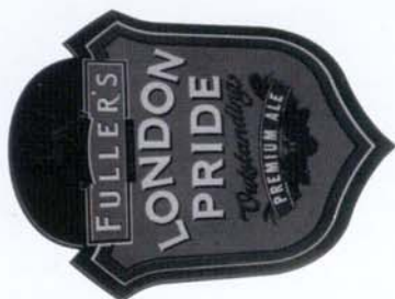
THE LONDON PRIDE LOGO WAS INSPECTED WITH AN AREA SCAN CAMERA AND BACKLIGHTING; A PINHOLE WAS DETECTED
