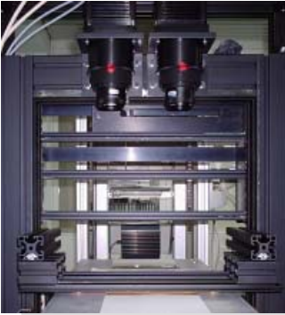
Inspection module (housing removed) with 2 line cameras
