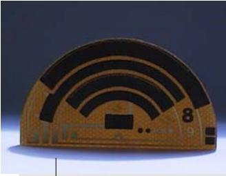
Inspection object with four concentric resistor tracks
